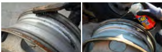
<Retirez la corrosion>
