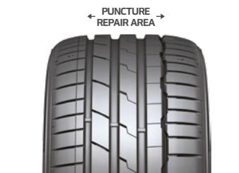
Repairs should only be made in the tread area (puncture repair area). None of the repair should extend into shoulder area. Puncture must be 1/4 inch (6mm) or smaller in diameter. Plug/stem and patch combination is only proper repair method. Repairs cannot overlap. Never repair an existing improper repair or tire worn down to 2/32nds of an inch. Contact Hankook Tire Technical Services for any repair on non-conventional tires (eg. Runflat, foam-lined)
